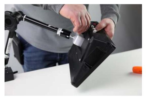
Option 2 is for mounting to a gooseneck mounting system with a  $\frac{1}{4}$ -20 threaded female socket. Attach your device's mounting tray to the adapter and secure with the two Phillips head screws. Thread the adapter with the  $\frac{1}{4}$ -20 screw into your gooseneck. Place your device into the mounting tray and press down to lock in place. See photos.
