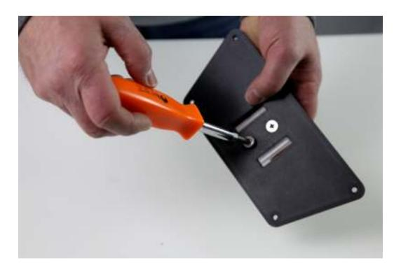
Next you will need to attach the mounting plate to the back of your Communication Builder. Use the included 4 long Philips Head screws. Please note the orientation of the mounting plate. It the screws will only line up one way as shown in the photo.
