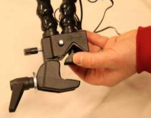
2. You can also remove one of the Easy Flex Dual Ultimate Switches from the clamp if only one switch is needed. To do this loosen the set knob on the clamp, then depress the spring loaded pin and lift up on the Flex arm to remove the switch from the clamp. See photos below.
