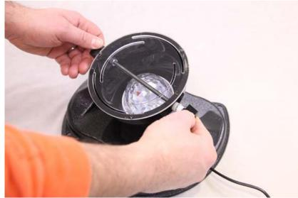
3. To activate the Sensory Projector, turn the ON/OFF toggle switch to ON. There is also an adjustable speed control knob. Clockwise increases the speed of the lights and counter-clockwise decreases the speed. When finished using the Sensory Projector turn the unit OFF.
