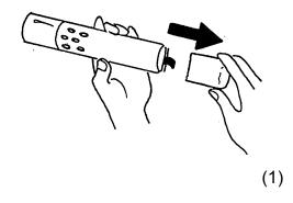
2. Expose the battery compartment on the fan assembly by pulling on the black tab. You only need to pull the fan assembly out half way to expose the battery case.
