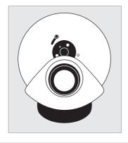
The [OPTI] Aura has been designed to accommodate 4" and 6" effect wheels. For 6" effect wheels the slide on the left of the magnetic adaptor should be at the top as per the image left.
