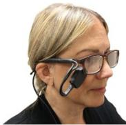
**Eye Blink Switch (#9008)** – A 7-year-old boy was paralyzed from the chin down in a car accident. Therapists at his rehab hospital contacted us about creating an eye blink switch so the boy could communicate using the switch and a scanning communicator.
